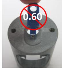
Angular bore: using jet gauge set (ROTAX part no. 281920) it must not be possible for plug gauge 0.60 mm to fit (picture left).
