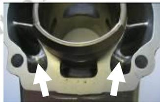
**12.5.7.2** All ports have chamfered edges (see picture right). Any additional machining is not permitted.
