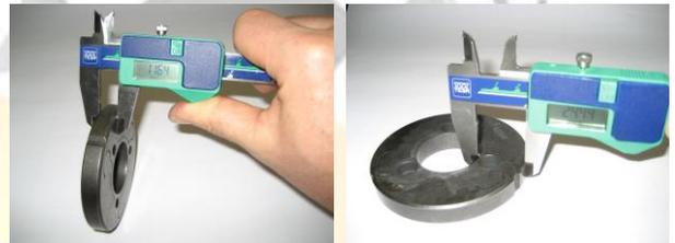
**13.4.3.3** Minimum outer diameter of clutch drum 89.50mm (picture near right)
