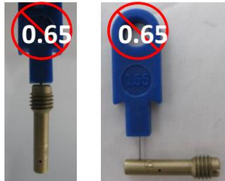
**13.8.15 Idle emulsion tube 60:** using jet gauge set (ROTAX part no. 281920) it must not be possible for plug gauge 0.65 mm to enter the bore (picture far left).
