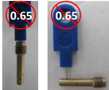
**11.6.15 Idle emulsion tube 60:** using jet gauge set (ROTAX part no. 281920) it must not be possible for plug gauge 0.65 mm to enter the bore (picture far left).
