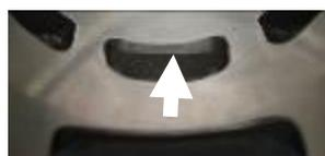
On cylinders marked 613933 the upper edge of the central boost port may show factory machining (see picture left).
