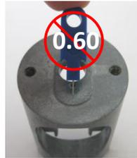
Angular bore: using jet gauge set (ROTAX part no. 281920) it must not be possible for plug gauge 0.60 mm to fit (picture left).
