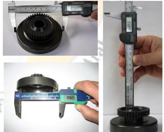
**13.4.3.5** Minimum height of sprocket with clutch drum assembly 39.50mm (picture far right).
