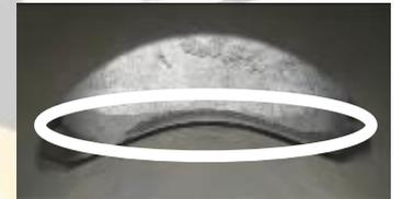
The exhaust ports of cylinders 223993 & 223994 may show factory machining all around.
