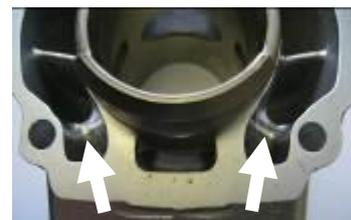
**10.5.7.2** All ports have chamfered edges (see picture top right). Any additional machining is not permitted.
