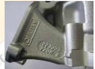
**10.5.6** Height of cylinder must be 87mm  $-0.05/+0.1$ mm (see picture right).
