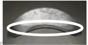
**12.5.8** The "exhaust port timing" (distance from the top of the cylinder to the top of the exhaust port) must be checked by means of the template (ROTAX part 277397).
