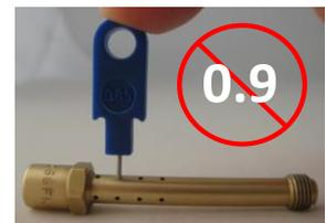
**13.8.14 Idle jet 60:** using jet gauge set (ROTAX part no. 281920) it must not be possible for plug gauge 0.65 mm to enter the bore of idle jet 60 (picture right).
