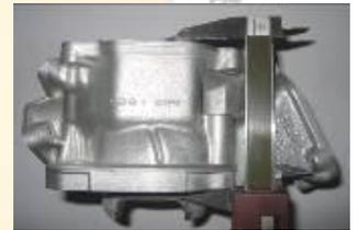
**12.5.7.1** All transfer ports and passages have cast finish surface except some removal (done by the manufacturer) of cast burr at the inlet passage and exhaust port and passages. All ports have chamfered edges to prevent ring snagging. Any additional machining is not permitted. The top edge of exhaust port may show some pre-existing machining from the manufacturer. The sealing flange for the exhaust socket may show signs of machining from the manufacturer (see picture right).
