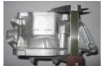
**10.5.7.1** All transfer ports and passages have cast finish surface except some removal (done by the manufacturer) of cast burr at the inlet passage and exhaust port and passages. All ports have chamfered edges to prevent ring snagging. Any additional machining is not permitted. The top edge of exhaust port may show some pre-existing machining from the manufacturer. The sealing flange for the exhaust socket may show signs of machining from the manufacturer (see picture right bottom).
