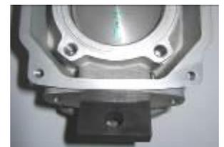
**10.5.9.2** Modifying the exhaust valve gasket (part no. 250 231) is illegal.
