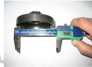
**11.4.3.5 Minimum height of sprocket with clutch drum assembly 33.90mm** (picture far right).
