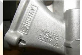
**12.5.6** Height of cylinder must be 86.7mm  $-0.05/+0.1$ mm (see picture right).
