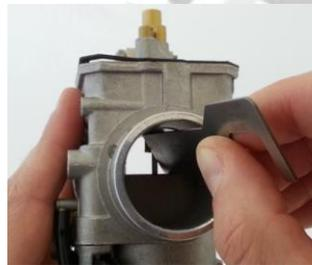
**A3.1.4** The cap of the carburettor must be screwed completely onto the carburettor (tight).
