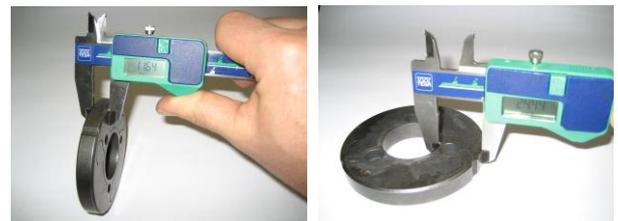
**11.4.3.3 Minimum outer diameter of clutch drum 89.50mm** (picture near right)
