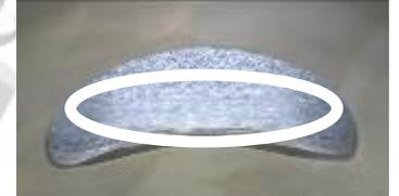
The exhaust port may show partial manual grinding done by the manufacturer to eliminate minor casting defects and to eliminate the NIKASIL burr at the end of the NIKASIL plating.
