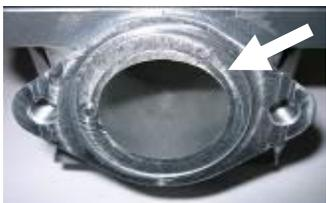
**12.5.7.4** The top edge of the exhaust port may show either just a cast finish surface (*picture below left*) or signs of a CNC machining (*picture below centre*) or signs of CNC machining in combination with signs of manual grinding (*picture below right*).
