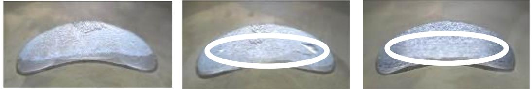
The exhaust port may show partial manual grinding done by the manufacturer to eliminate minor casting defects and to eliminate the NIKASIL burr at the end of the NIKASIL plating.
