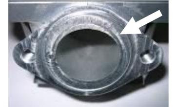
**10.5.7.4** The top edge of the exhaust port may show either just a cast finish surface (picture below left) or signs of a CNC machining (picture below centre) or signs of CNC machining in combination with signs of manual grinding (picture below right).
