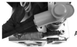
(A) additional ground cable not connected
