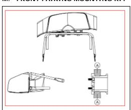
THE FRONT FAIRING IS NOT IN AN ACCEPTABLE POSITION IF ANY PART OF THE TUBES OF THE FRONT BUMPER ARE IN THE AREA 'A'.
