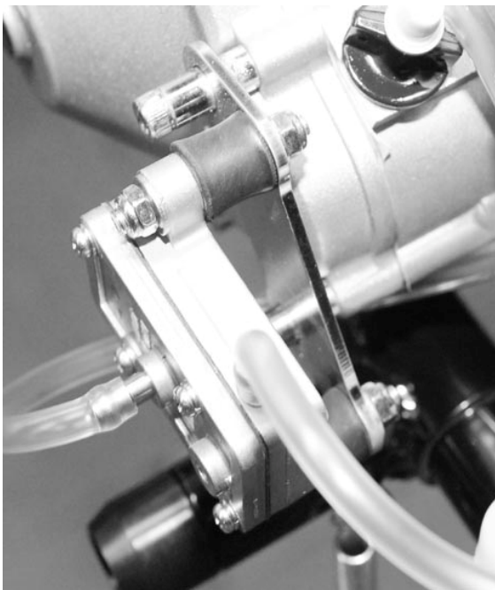
Foto of the frame with the section of the support for the fuel pump (fuel pump mounted)
